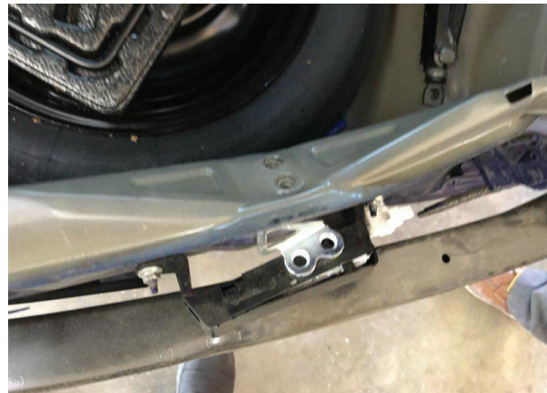
Frame damage from the impact to the Noriega car.
