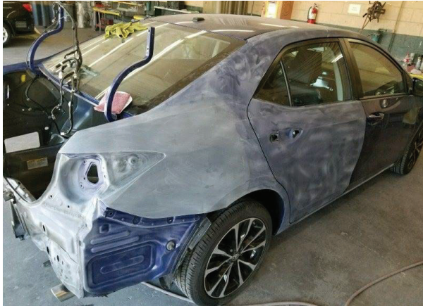
The Noriega car in the body shop, mid-repair. The impact was heavy enough to damage the trunk lid, the rear quarter panel, and the rear passenger-side door.
